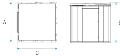
**The FEKO+ waste water receipt station** is a multifunctional device for collecting municipal and industrial wastewater. The device identifies carriers, wastewater suppliers, and also measures and controls the parameters (pH, temperature) and quantity of the delivered wastewater. It is possible to block the admission of wastewater in which measurement transducers have detected exceedances (e.g. pH) established in the FEKO+ programme dedicated to the catchment station.
