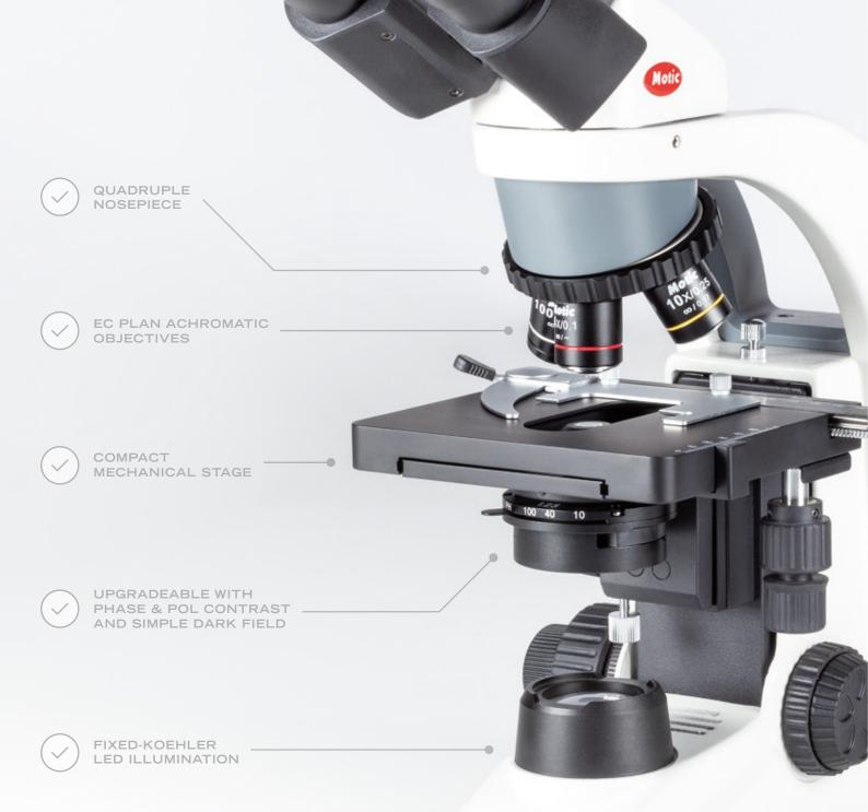
in a Fixed-Koehler setup gives adequate power resources for upgrading the microscope with contrast methods like Phase contrast, Polarization or Darkfield. The Motic BA210 is a robust student instrument that brings professional, repeatable image results from all intended applications.
